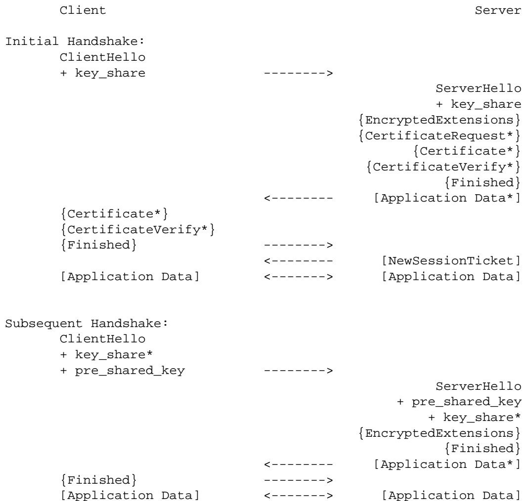
Figure 3: Message flow for resumption and PSK
