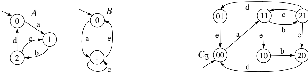
FIGURE 1. LTSs A and B , and the composite machine C_{\mathfrak{S}} of system \mathfrak{S} = A \parallel B .
